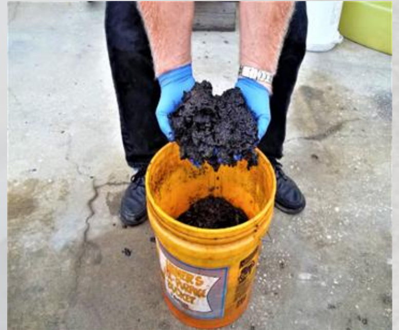
Plugged fuel filter caused by bio-mass & microbe excreted waste
