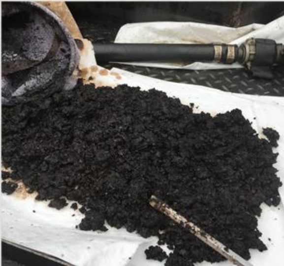
Asphaltenes removed from tank bottoms developed due to unstable fuel
