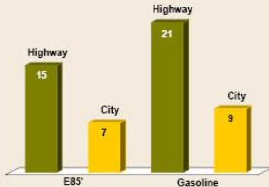
Fuel Economy of a Chevrolet Tahoe Using Gasoline and Ethanol (miles per gallon)
