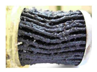
It is a fact that 70% of all diesel engine break downs are caused by fuel system-related problems. In many cases the problems are caused by fuel contaminated with bacteria, fungus or mold. The residue created by these nasty little bugs plugs fuel filters, which causes difficulties with starting, poor acceleration, stalling and no-start conditions.
