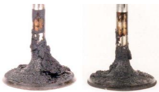
Deposits on valve stems
