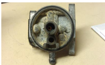
Ethanol solvency deposits accumulated in a small engine carburetor
