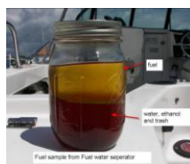
Ethanol sludge from a fuel tank
