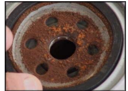
Corroded Fuel Filter
