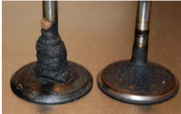
This picture shows one of the final destinations for resin dissolved by ethanol-blends
