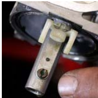
Plugged Fuel Jet
