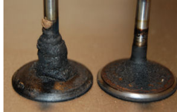
Buildup of ethanol-dissolved resin on valve stems
