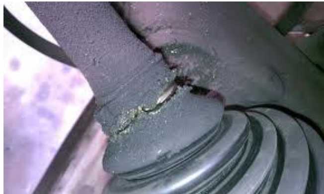
Damaged CV Boot. If this is not repaired, the grease will leak and destroy the CV axle
